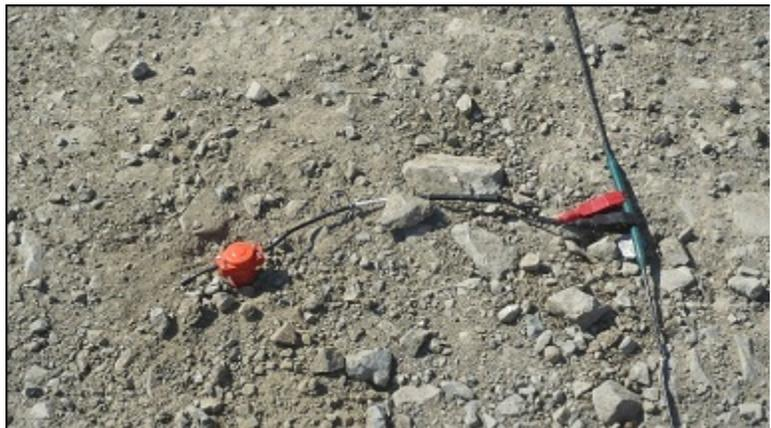
Figure C.1. Geophone installed in subsurface.
