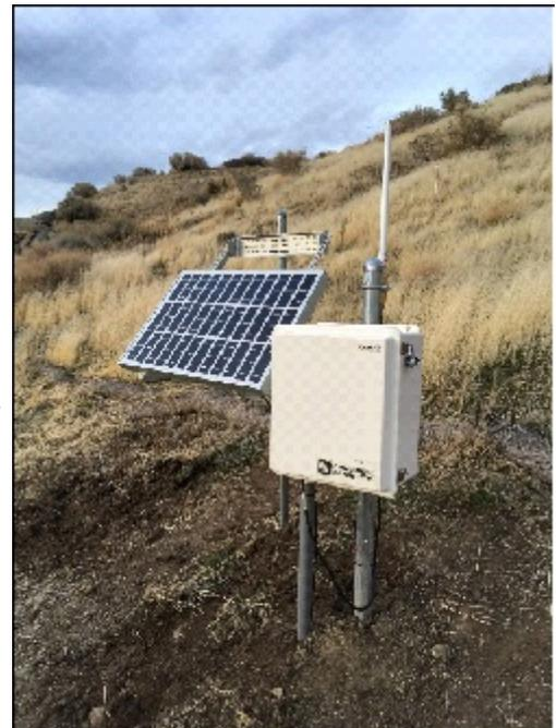
Figure C.4. Automated Data Acquisition System (ADAS) similar to the systems to be installed in Montecito.
