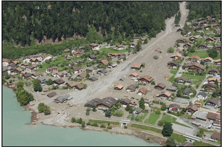
*Figure 16. Catastrophic damage to the town of Brienz, Switzerland in summer 2005 was similar to that experienced by Montecito after the January 9, 2018 debris flows.*
